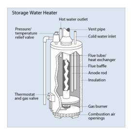
Conventional storage water heaters remain the most popular type of water heating system for the home. Here you'll find basic information about how storage water heaters work; what criteria to use when selecting the right model; and some installation, maintenance, and safety tips.
